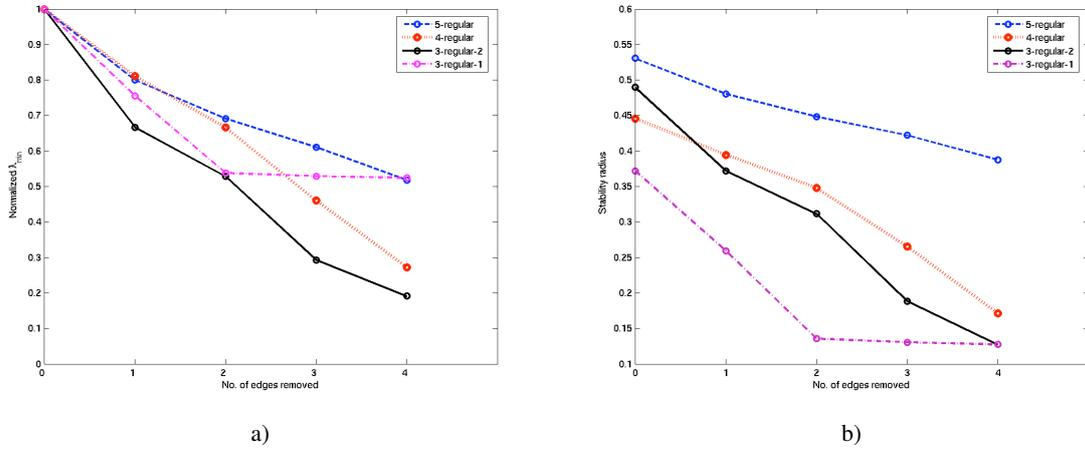
**Fig. 7.** a) Normalized minimal Laplacian eigenvalues for some communication link failures. b) The stability radii for some communication link failures.
