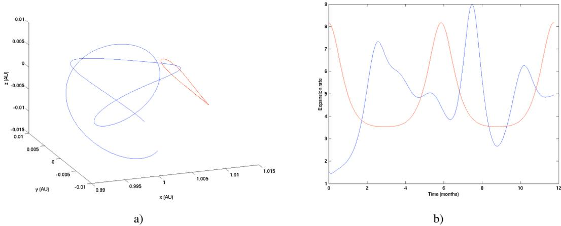
**Fig. 3.** a) Orbit w.r.t. initial condition chosen within the box having minimal expansion (blue) and Halo orbit as suggested in [10, 19] (red). b) Comparison of expansion rates along the two orbits (two periods of the Halo orbit).
