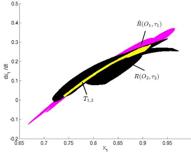
Figure 3. Intersection  $\mathcal{T}_{1,2}$  (light grey) of two reachable sets in a common intersection plane.  $\hat{\mathcal{R}}(\mathcal{O}_1, \tau_1)$  (dark grey): reachable set of the gateway set of the Earth,  $\mathcal{R}(\mathcal{O}_2, \tau_2)$  (black): reachable set of the gateway set of Venus. The figure shows a projection of the covering in 3-space onto the  $(x_1, \dot{x}_1)$ -plane (normalized units).
