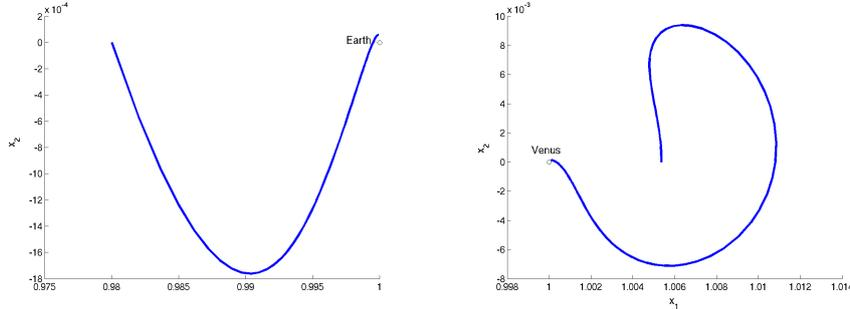
(a) From Earth to the gateway set  $\mathcal{O}_1$ , control force  $-700$  mN, flight time 0.1 years,  $\Delta V = 630$  m/s. (b) From the gateway set  $\mathcal{O}_2$  to Venus, control force  $-9$  mN, flight time 0.27 years,  $\Delta V = 20$  m/s.
