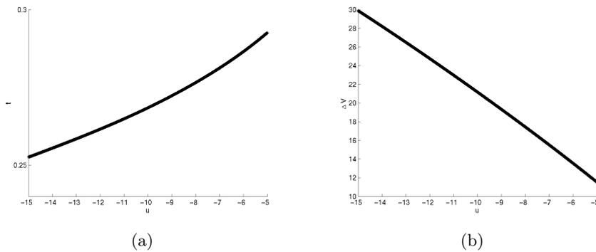
Figure 6. Transfer time  $t$  (years) and  $\Delta V$  (m/s) in dependence of the applied control force  $u$  (mN) for the transit from the gateway set  $\mathcal{O}_2$  into a neighborhood of Venus.
