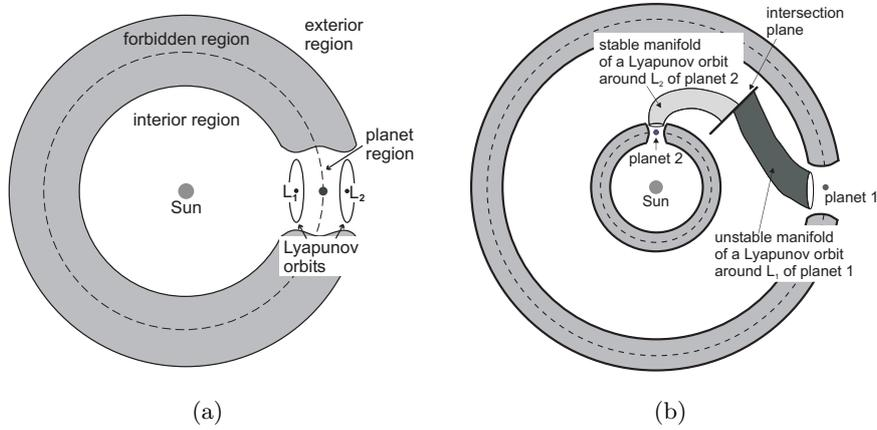
Figure 1. (a) Projection of an energy surface onto position space (schematic) for a value of the Jacobi integral for which the spacecraft is able to transit between the exterior and the interior region. (b) Sketch of the ‘‘coupled 3-body approach’’ (cf. (Koon et al., 2000b, Koon et al., 2002)). The idea is to travel within certain invariant manifold ‘‘tubes’’ possibly including an impulsive maneuver at the intersection plane.
