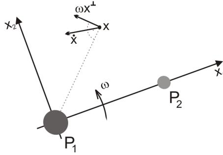
Figure 2. The velocity of the spacecraft with respect to the inertial frame is given by  $\dot{x} + \omega x^\perp$ .
