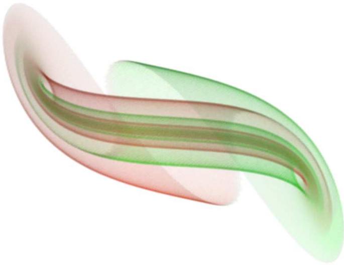
Figure 10: Volume rendering of Chua's circuit with different coloring for two almost invariant subsets. The red, respectively blue coloring indicates subsets in which trajectories stay for a very long time until they turn over to the other subset.
