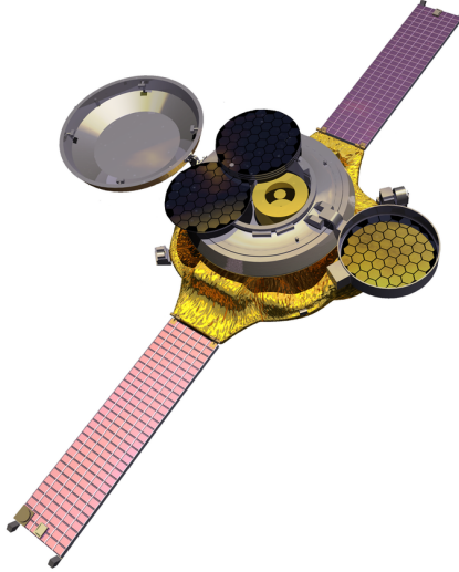
Figure 1: The Genesis spacecraft as it faces the sun to collect particles of solar wind while orbiting L_1 .
