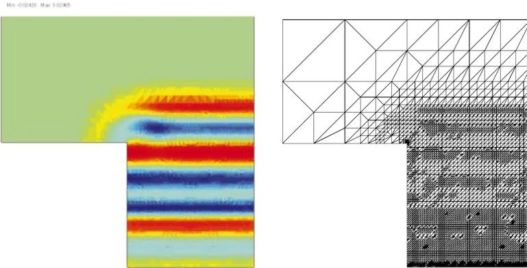
**Fig. 3.** Solution and triangulation for time-step # 20,  $t = 0.27$ , (Example 2). Notice that the upper boundary of the initial perturbation was located at  $x_2 = 0.4$ . The *color-coding* is chosen as follows: the green of the upper left corner belongs to zero, the maximum negative value is dark blue, the maximum positive value dark red. In between, the colors are distributed as in the spectrum of visible light.
