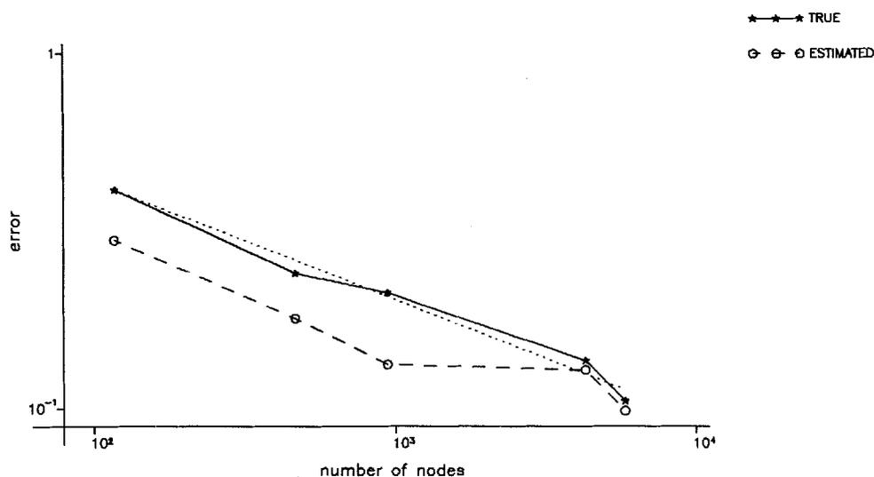
Figure 13. Discretization error and *a posteriori* error estimation
